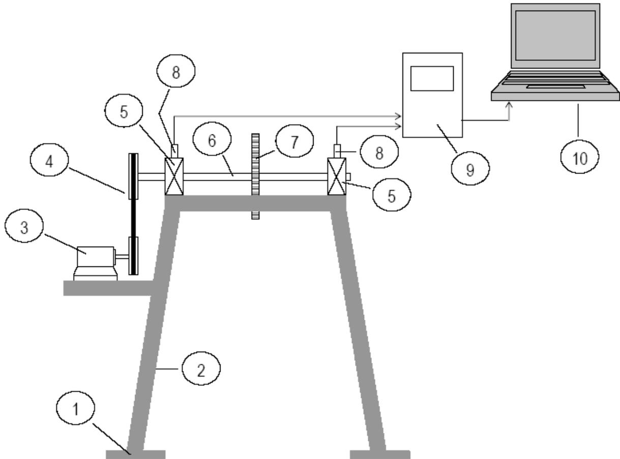
Figure 1. Experimental set up of rotor-bearing system
