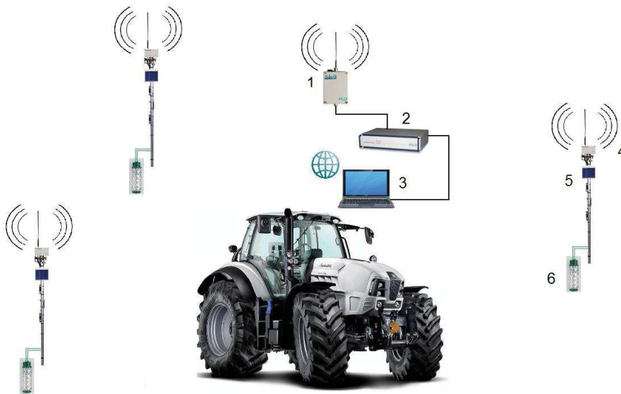
Fig. 1. Remote monitoring of soil moisture from an agricultural tractor: (1) Wireless modem, (2) Gateway, (3) Laptop Computer, (4) Remote Terminal Unit, (5) Solar Panel, and (6) Soil moisture Sensor.
