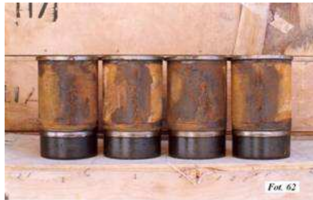
Figure 3: Corrosion and cavitation erosion in wet-sleeve liners was observed after 1000 working hours. It is about a turbocharged engine with 4 cylinders of bore x stroke = 105 x 115,5 mm, in the cooling system of which anticorrosion and anticavitation inhibitors had not been used.
