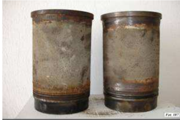
Figure 5: Wet-sleeve liners were not damaged by cavitation erosion after 5600 h operation. This approach was tested on a turbocharged engine with 6 cylinders of bore x stroke = 110 x 120 mm. The thickness of the liner wall was 8,3 mm, and the cooling system is not properly maintained.
