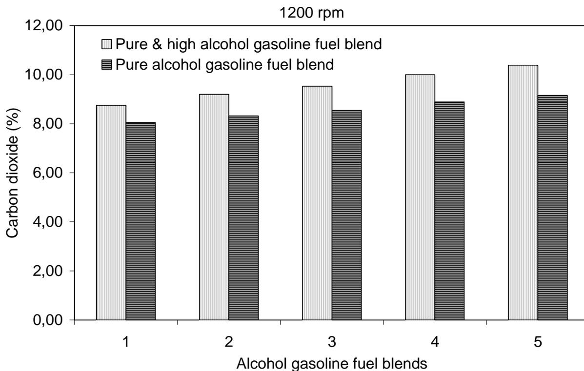
Figure 7: Comparison of CO<sub>2</sub> exhaust emission between pure-high alcohol/gasoline and pure alcohol/gasoline fuel blend at 1200 rpm.
