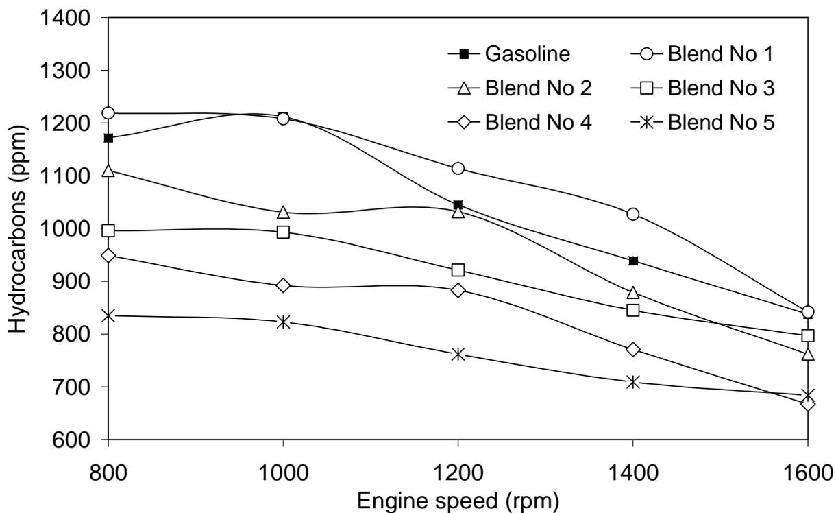
Figure 4: The variation of Hydrocarbons (HC) emissions in relation to the engine speed.
