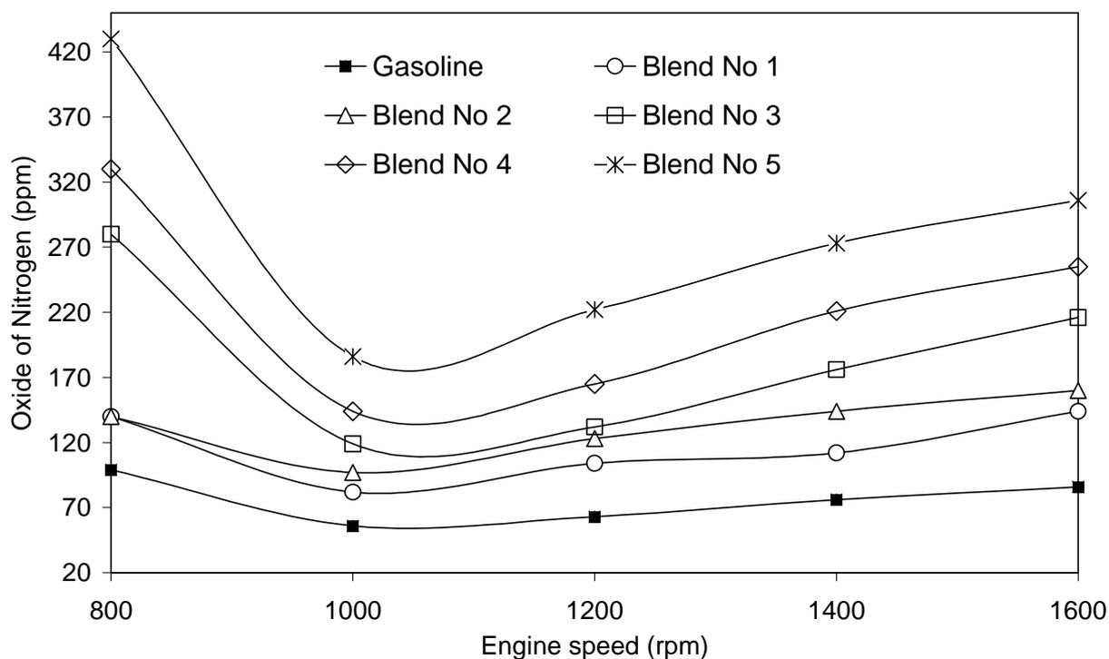
Figure 5: The variation of Oxide of Nitrogen (NO) emissions in relation to the engine speed.
