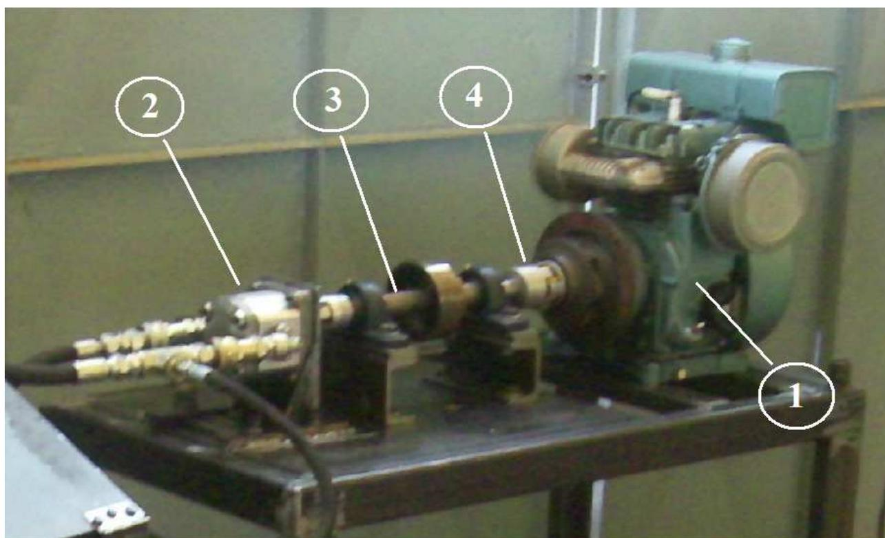
Figure 1: Photograph of the experimental set-up. 1-Engine, 2-Dynamometer, 3-Shaft, 4-Flywheel.
