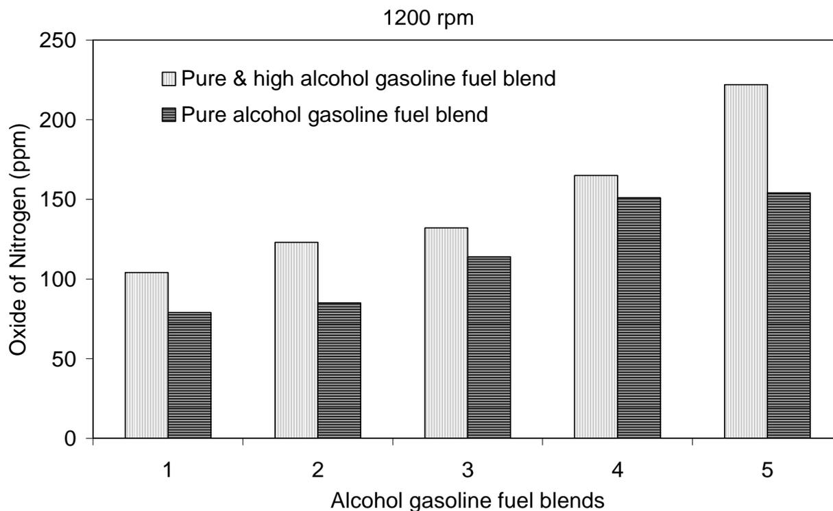
Figure 9: Comparison of NO exhaust emission between pure-high alcohol/gasoline and pure alcohol/gasoline fuel blend at 1200 rpm.
