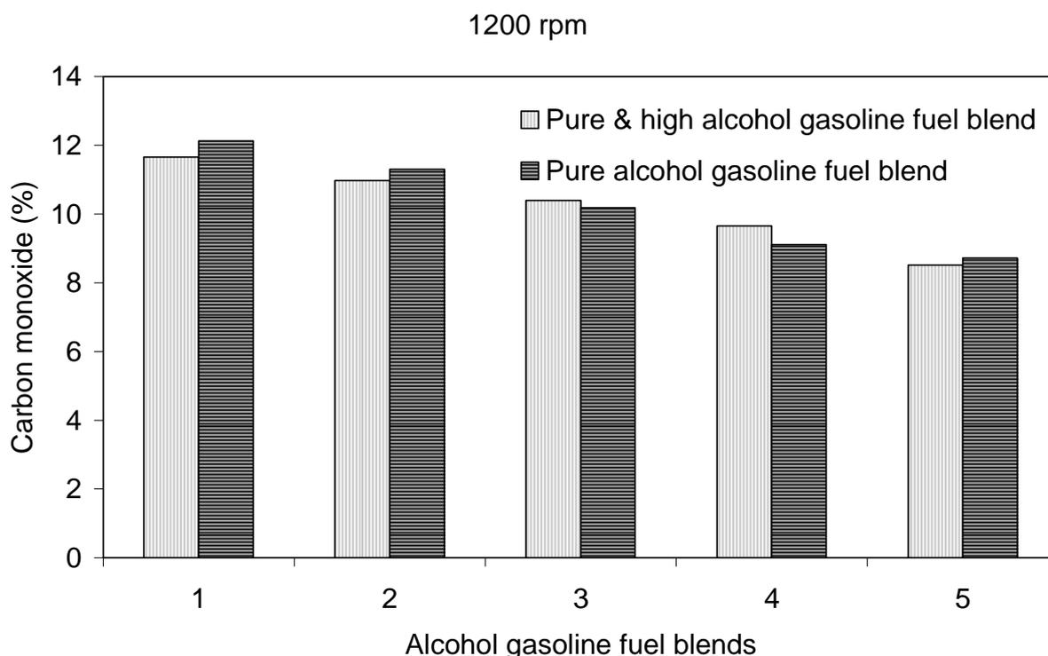
Figure 6: Comparison of CO exhaust emission between pure-high alcohol/gasoline and pure alcohol/gasoline fuel blend at 1200 rpm.
