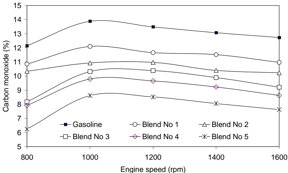
Figure 2: The variation of Carbon monoxide (CO) emissions in relation to the engine speed.
