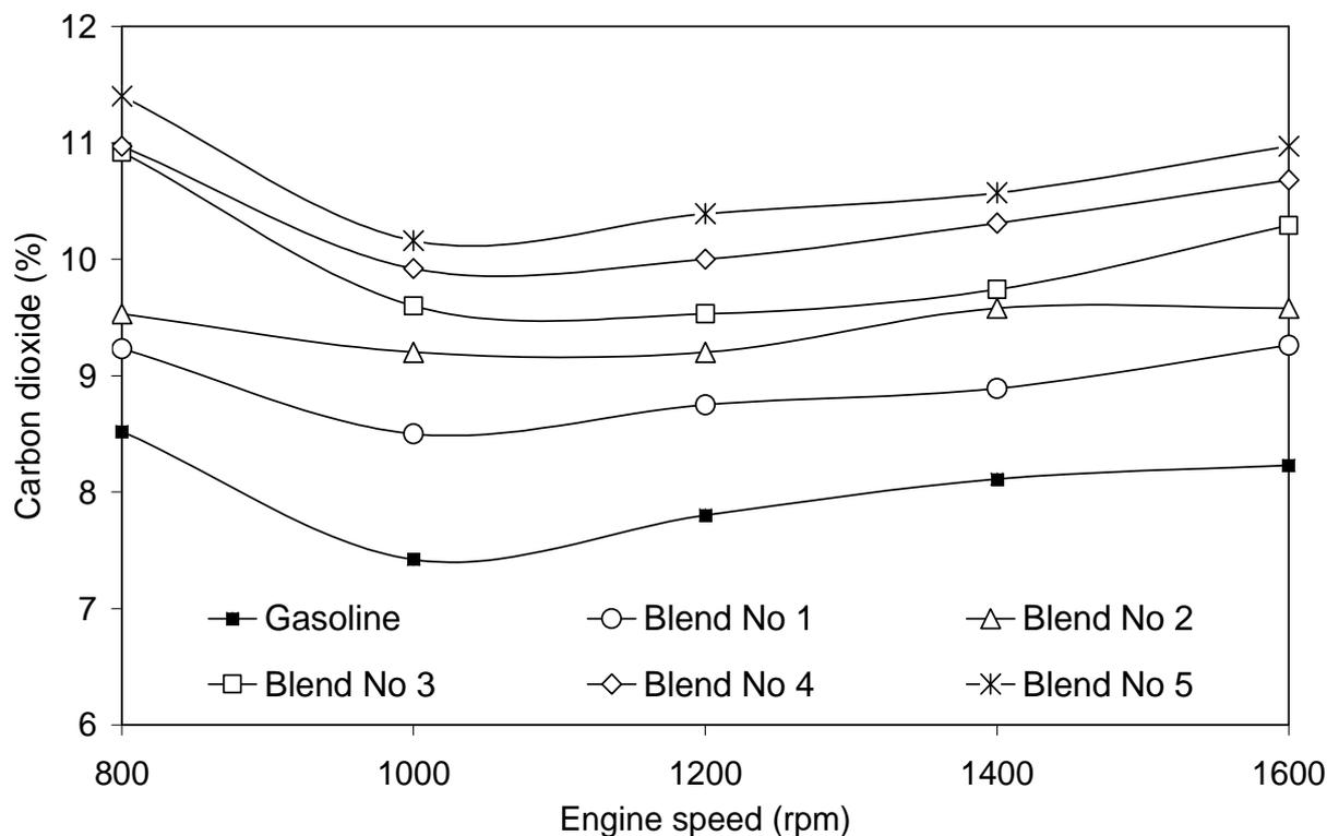
Figure 3: The variation of Carbon dioxide (CO<sub>2</sub>) emissions in relation to the engine speed.
