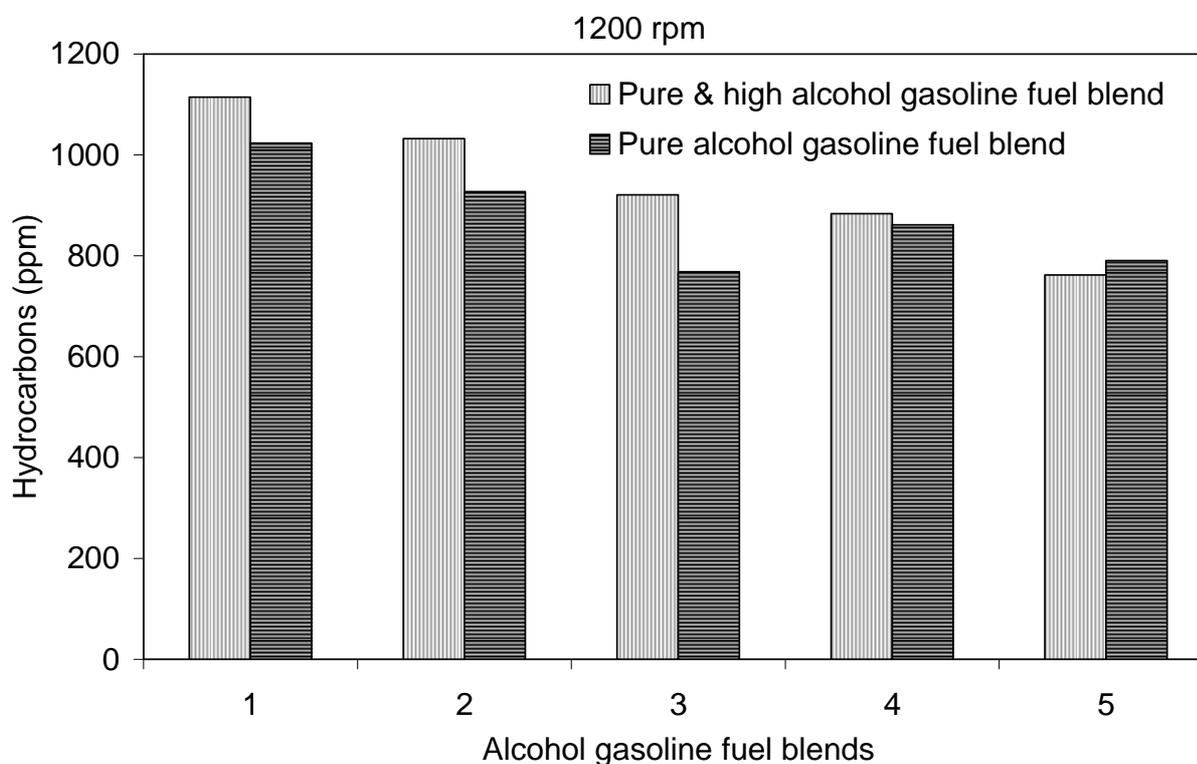
Figure 8: Comparison of HC exhaust emission between pure-high alcohol/gasoline and pure alcohol/gasoline fuel blend at 1200 rpm.
