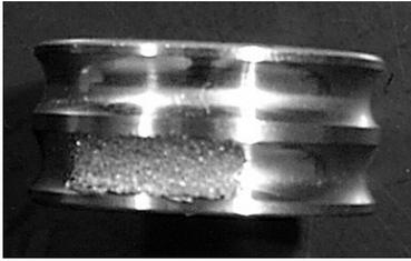
Figure 1. Example of an extended fault in the inner race
