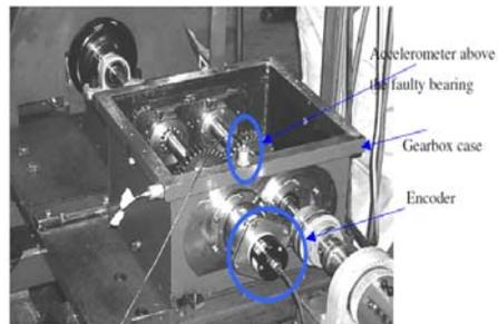
Figure 2. The spur gear rig
