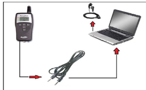
Figure 3. Data acquisition setup for sounds emitted from malfunctioning injectors. The Bearing Checker (by SPM Instrument) is shown on the left.
