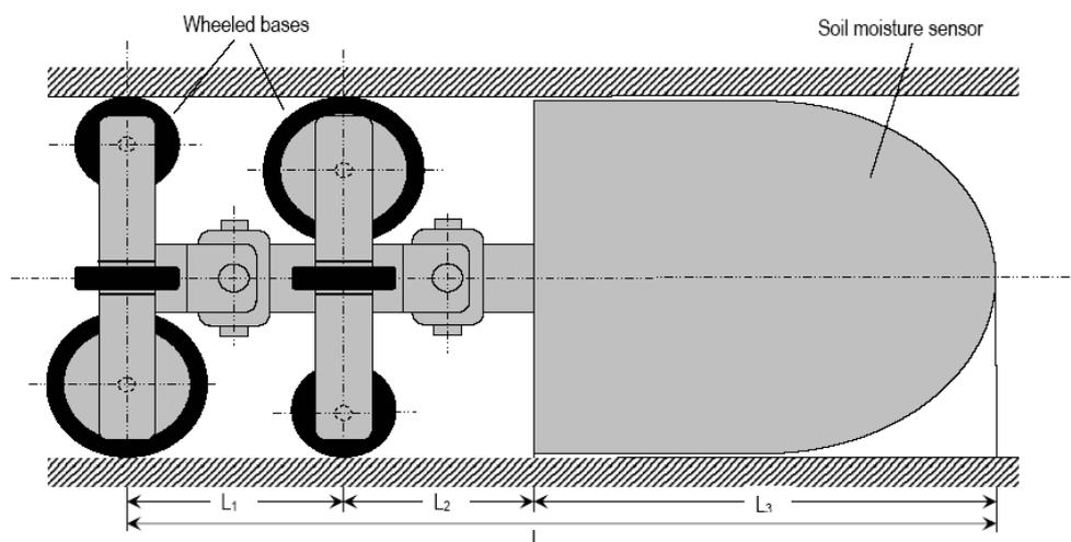
Fig. 1: The mechanical drawing of the mobile platform that monitors soil moisture.
