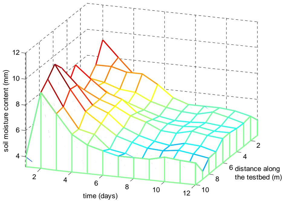
*Fig. 5: Soil moisture changes along the experimental testbed at a depth of 10 cm after furrow irrigation method.*
