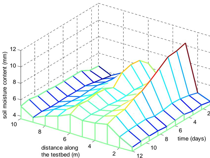
Fig. 8: Soil moisture changes along the experimental testbed at a depth of 10 cm after drip irrigation method.
