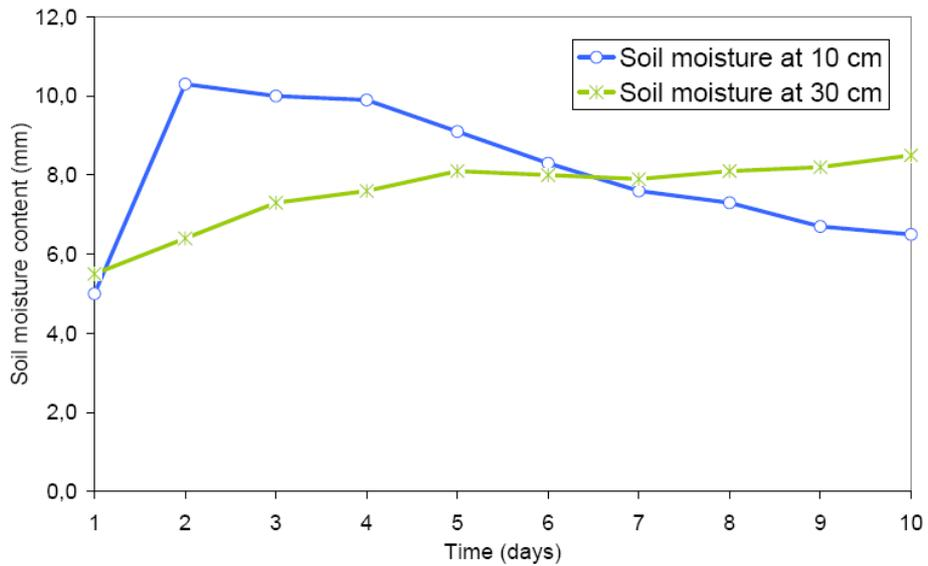
Fig. 7: Soil moisture changes in soil profile of the experimental testbed after drip irrigation method.
