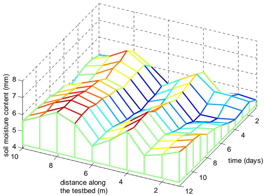
*Fig. 6: Soil moisture changes along the experimental testbed at a depth of 30 cm after furrow irrigation method.*
