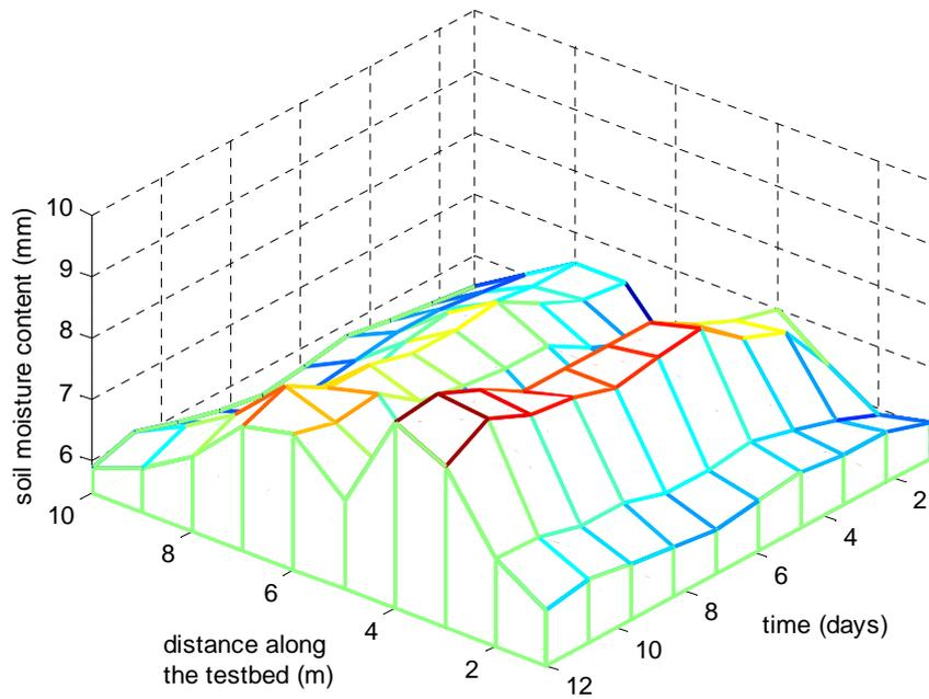
Fig. 9: Soil moisture changes along the experimental testbed at a depth of 30 cm after drip irrigation method.
