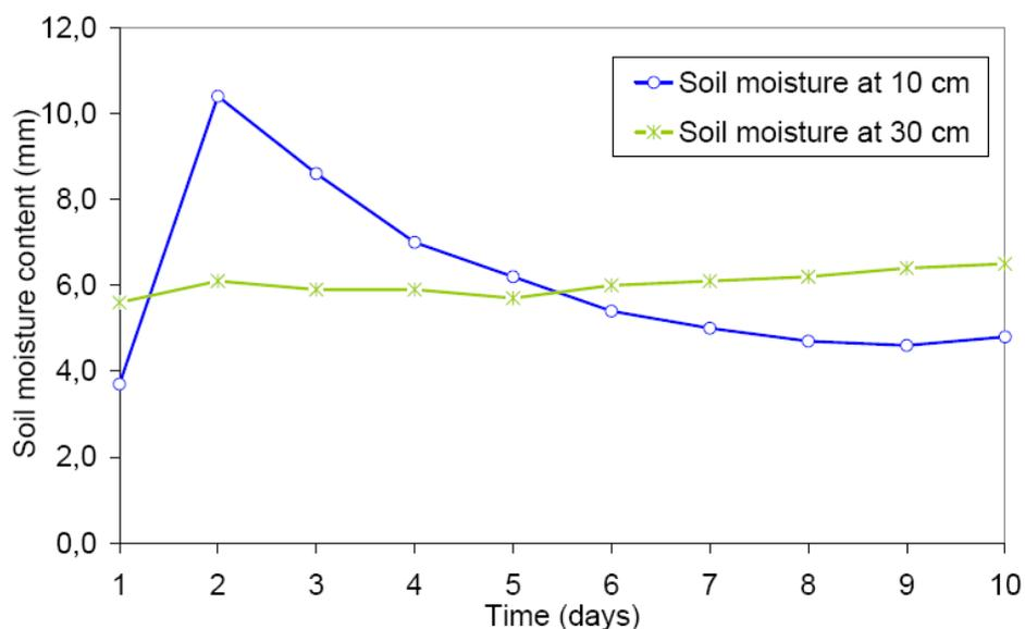
*Fig. 4: Soil moisture changes in soil profile of experimental testbed after furrow irrigation method.*
