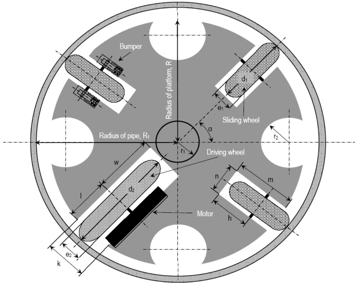
Fig. 2: The mechanical drawing of the circular wheeled base.
