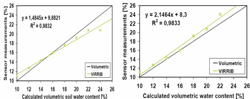
Figure 4 - Comparison of volumetric soil water content as determined by Virrib Sensor and from calculated volumetric content: a) in loam and b) in sandy loam.
