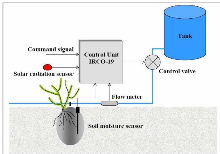
Figure 1 - Block diagram of automated control system.
