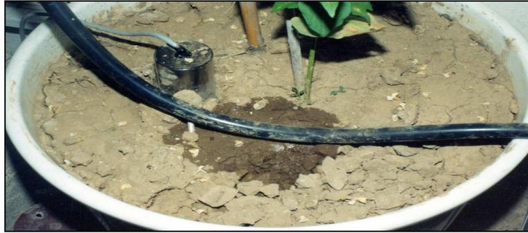
Figure 3 - Soil moisture sensor Virrib under laboratory conditions.
